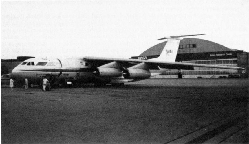
The Kuiper Airborne Observatory (KAO) is a converted C-141 transport plane used for observing at an altitude of 12.5 kilometres. Photo by Neil Rowlands.
