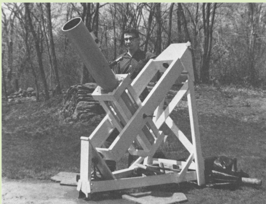
Fig. 3—A 6" reflector is easily carried by this yoke mounting. The extra long tube shields the optics for deep sky observation. The same mount carried an 8" f/10 reflector for several years.
