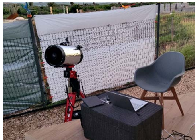
Figure 2 – Final setup with wind tarps in place. Tripod was set low, to keep the telescope below the top of the tarps.
