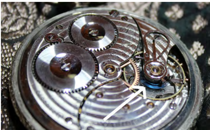
Figure 4 — Photograph of a late 19th-century railway chronometer movement by American Waltham; the arrow points to the blue-steel watch spring, to illustrate the colour William Huggins cited. Reproduced courtesy of the Specula Astronomica Minima.
