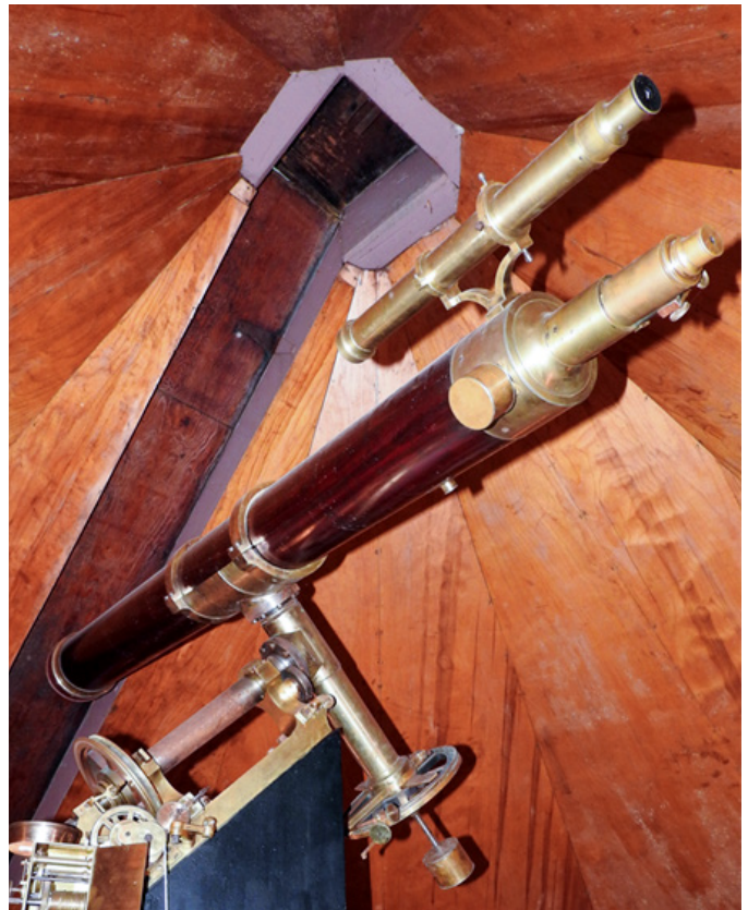
Figure 5 — The 175-year-old 15-cm f/11 refractor by Merz seen inside the beautiful octagonal dome of William Brydone Jack Observatory, UNB. (Larry Dickinson, MyNewBrunswick.ca )
