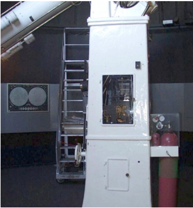
Figure 2 — 15-inch pier, showing nitrogen tank to dry the Perkin-Elmer apo lens, Credit: CMST collection — Warner & Swasey Co., Telescope, circa 1905, artifact no. 1974.0488.001, Ingenium — Canada’s Museums of Science and Innovation, http://collection.ingeniumcanada.org/en/item/1974.0488.001/
