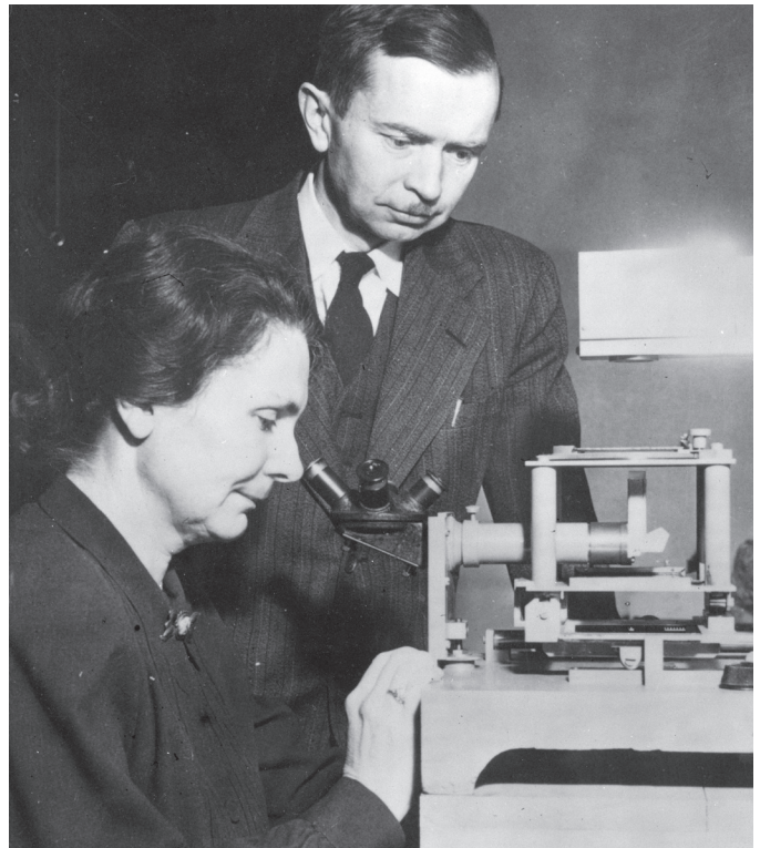
Figure 3 — Helen Sawyer Hogg working with a blink microscope. This is the device she used for discovering globular cluster variable stars on photographic plates. Her husband Frank is looking on. Credit: University of Toronto Archives - B1994-0002/005P (08)
