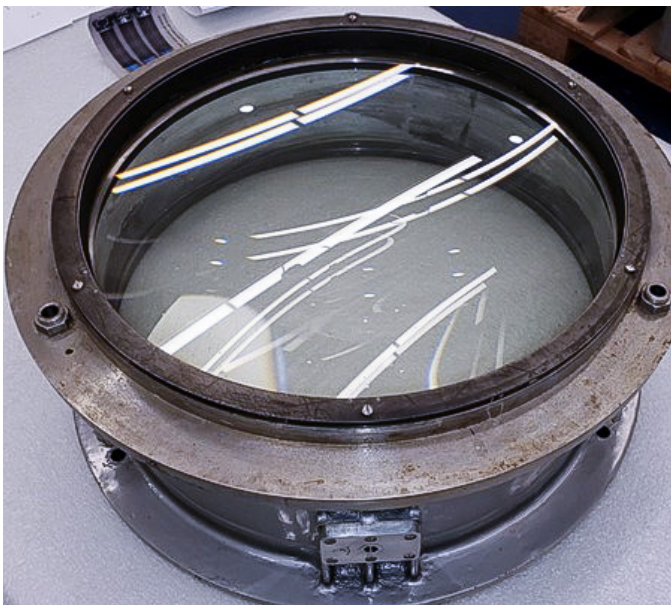
Figure 4 — 15-inch Perkin-Elmer triplet apo lens and cell, showing multiple reflections of ceiling fluorescent lights from the uncoated elements. Photo by James Gort, courtesy of Canada's Museum of Science and Technology.
