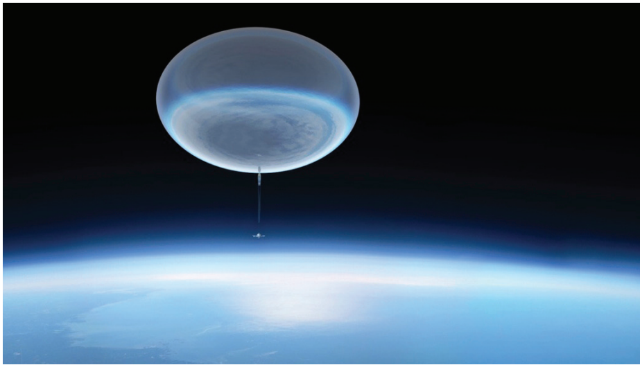
Figure 5 — An illustration showing an ASTHROS high-altitude balloon ascending into the stratosphere. When fully inflated, these balloons are 150 metres wide and reach an altitude of 40 kilometres. Image: NASA Goddard Space Flight Center Conceptual Image Lab/Michael Lentz
