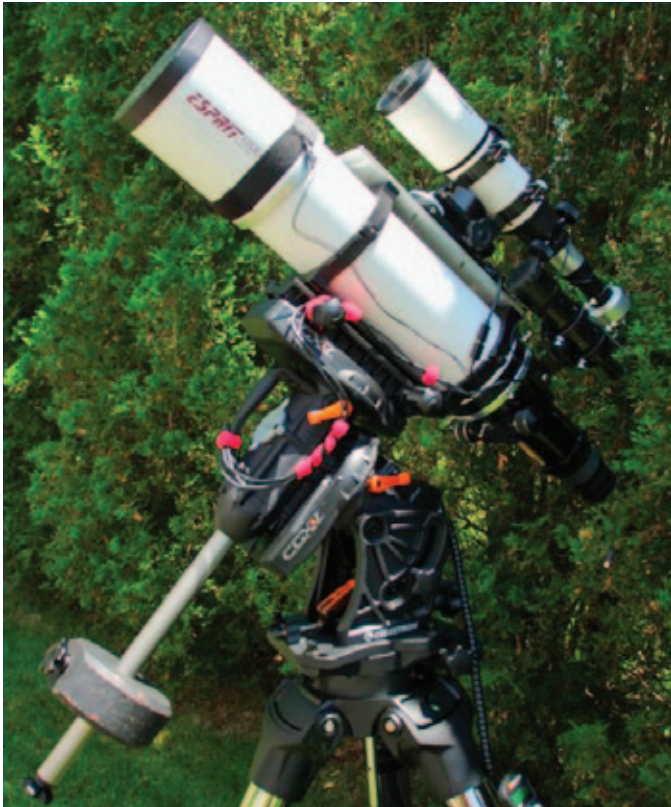
Figure 2 — My setup, note the cabling tied off the carrying handles with a loop to allow for motion of the declination axis.
