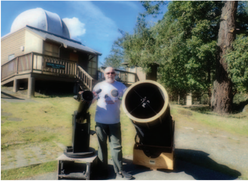
Figure 1 — The author at his favourite observing site with his 150-mm f/8 Orion Dob and his 500-mm f/3.3 Starmaster.
