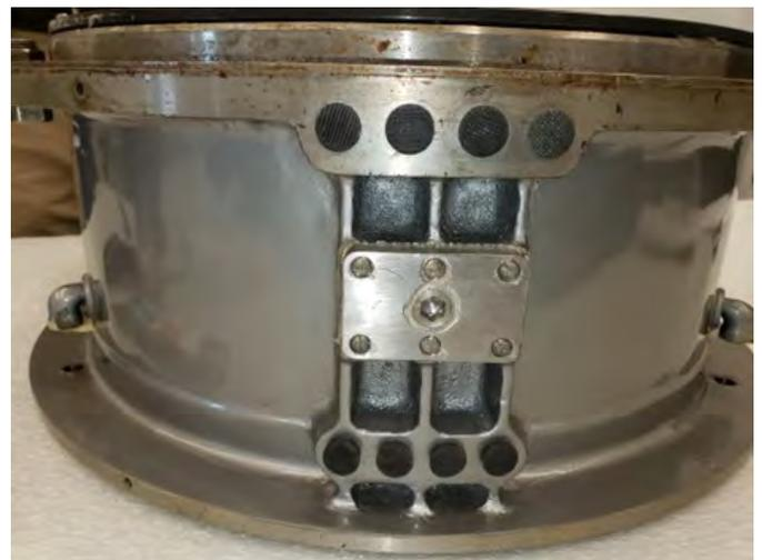
Figure 5 — Side view of the massive Perkin-Elmer lens cell. Photo by James Gort, courtesy of Canada’s Museum of Science and Technology.
