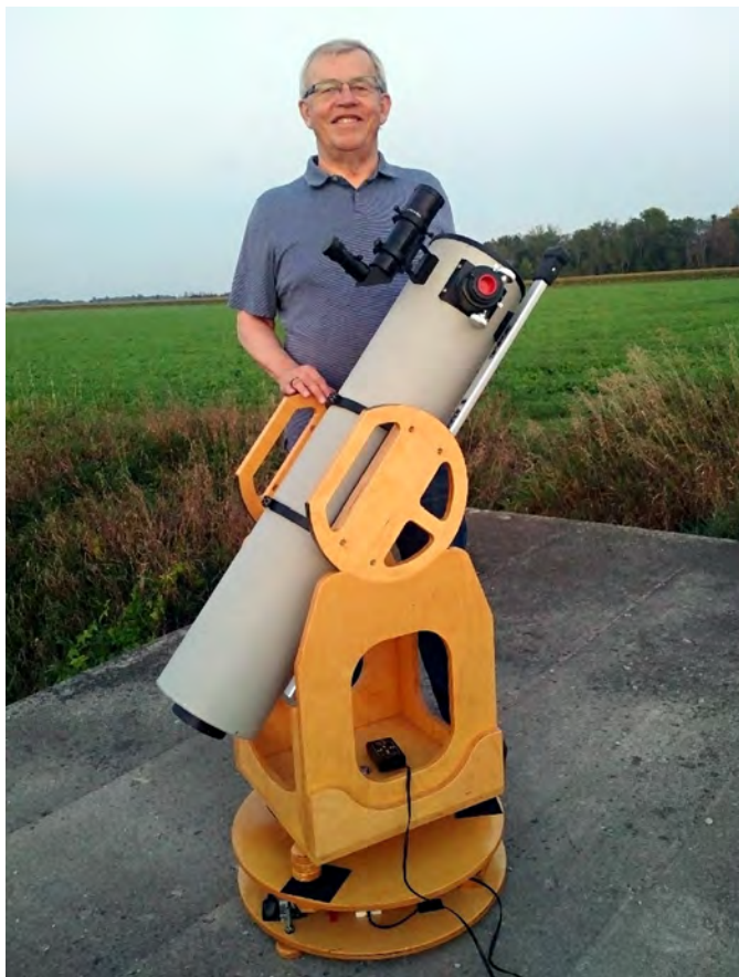
Figure 4 — Mount built by Peter Pekurar for Rudolph Dorner's Intes-Micro ALTER MN 76 (178-mm Maksutov-Newtonian).
