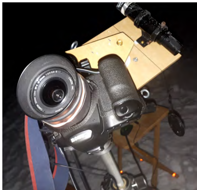
Figure 1 — DSLR with dew heater on barn door tracker. Yes, upside-down, for balance.
