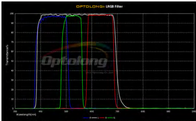
Figure 2 — Transmission characteristics of Optolong's LRGB filter set used in this experiment.
