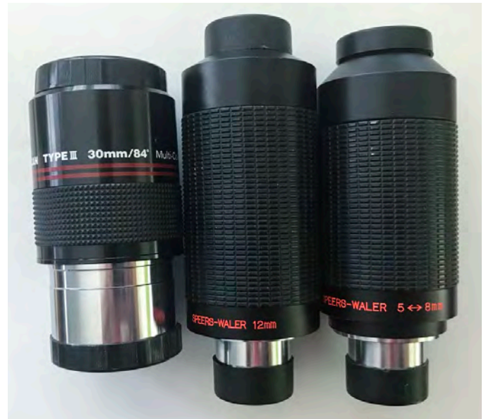
Figure 2 — Used set with a zoom eyepiece— a 30 mm, a 12 mm, and a zoom eyepiece. WALER = Wide Angle, Long Eye Relief, original design by Glenn Speers of Antares, no longer for sale on the retail market.
