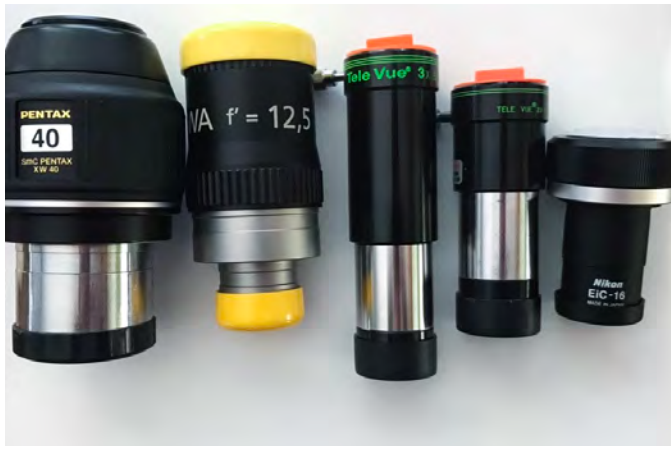
Figure 1 — My “minimalist” set now includes two eyepieces and three Barlows: a 40-mm wide-angle (70°); a 12.5-mm 84°, plus 1.6×, 2×, and 3× Barlows.
