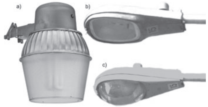
Figure 11 — Luminaires with different glare characteristics. The cut-off limits apply to the light that shines above the horizon and contributes directly to artificial sky glow. (a) The typical dust-to-dawn luminaire has very limited shielding. They are designed to scatter light at angles except directly upward. Less than 25% of the light illuminates the nadir. (b) Full Cut-Off fixtures can be identified by their “flat and horizontal window.” The recessed lamp prevents up-light and limits the emission within 10^\circ below the horizon to 10% of the total light output. (c) The “drop glass” cobra fixture is called a “Semi Cut-Off” —allowing up to 5% up light. A shallower lens, called a “Cut-Off”, allows 2.5% up light.
