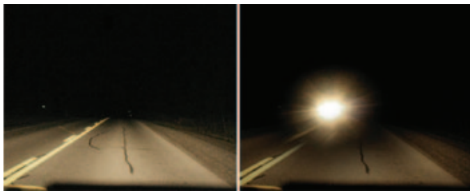
Figure 3 — View down a rural road with an approaching car. Although modern bright headlights provide illuminance to increase visibility for the driver who cannot see the luminance of their lights, the glare is debilitating for the opposing traffic.
