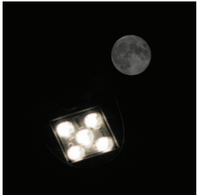
Figure 10 — Comparison of the luminance of the Moon to an LED street-light. The Moon illuminates the countryside to a maximum of about 0.1 lux (scotopic vision) with a luminance of only 4,000 cd/m 2 (4,000 nits). The small emitters in a LED fixture must illuminate a very large surface to levels suitable for our photopic vision (>3-lux) requiring a luminance of 100,000 to over a million nits.
