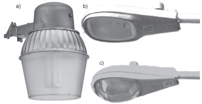
Figure 11 — Luminaires with different glare characteristics. The cut-off limits apply to the light that shines above the horizon and contributes directly to artificial sky glow. (a) The typical dust-to-down luminaire has very limited shielding. They are designed to scatter light at angles except directly upward. Less than 25% of the light illuminates the nadir. (b) Full Cut-Off fixtures can be identified by their “flat and horizontal window.” The recessed lamp prevents up-light and limits the emission within 10 degrees below the horizon to 10% of the total light output. (c) The “drop glass” cobra fixture is called a “Semi Cut-Off” —allowing up to 5% up light. A shallower lens, called a “Cut-Off”, allows 2.5% up light.
