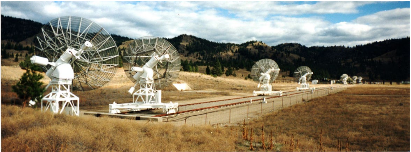
Fig. 2 — The DRAO Synthesis Telescope, seen from the west in 2000. Seven 9-metre equatorially mounted antennae stretch eastward along a 600-m baseline. (Someone vetoed naming them Happy, Sleepy, Dopey, Grumpy, Bashful, Sneezzy, and Doc.) Three are on wheels, for positioning along a 300-m track. Buried cables connect receiver front ends in the focus boxes to additional electronics and digital correlators in the concrete building near the middle of the array.
