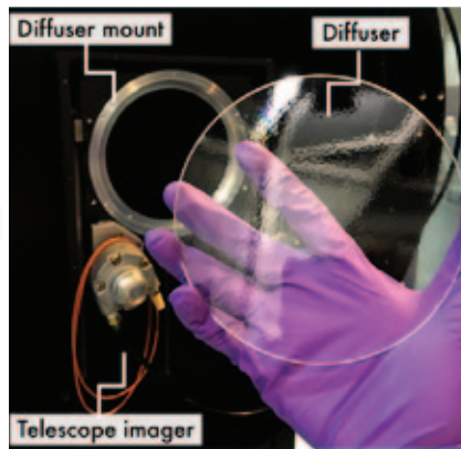
Figure 3 — Left: Light from a laser pointer is shaped into a wide and stable output using a beam-shaping diffuser. A carefully designed pattern is precisely molded into plastic polymers or directly into a glass substrate, creating micro-structures on the surface of the diffuser (credit: RPC Photonics). Right: The diffuser installed at the ARC 3.5-m telescope at Apache Point Observatory. Image Stefansson et al. 2017.
