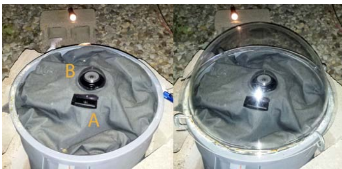
Figure 1 — The Zenith-SQM (A) and AllSky camera (B) inside their weather-proof housing, which is weighted down and reinforced against strong winds. The camera is level and oriented north and east. The SQM is mounted to the north side of the camera housing and points straight up. The photo on the right shows the Plexiglas weatherproof bubble that covers the instruments.
