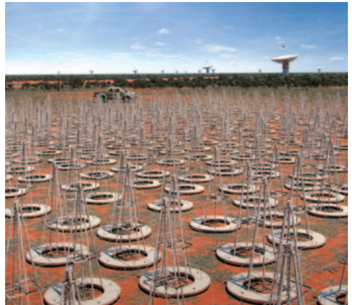
Figure 1 — Part of the Low Frequency Array component of the proposed Square Kilometre Array telescope. This part of the array would be sited primarily in the western part of Australia. The field of antennas is connected to a massive supercomputer, which produces images of the radio sky. New facilities would be well suited to conduct a thorough search of the radio sky for extraterrestrial signals. Image Credit: SKA Organization.
