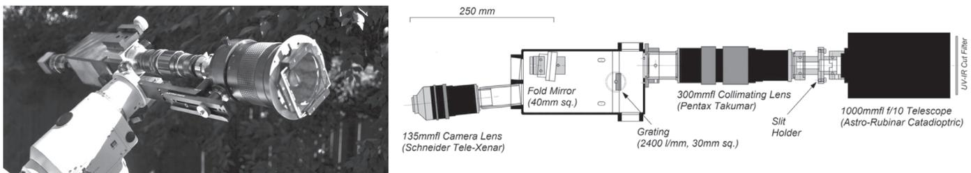
Figure 4 — Schematic diagram and photograph of the instrument. It is shown attached to an NEQ-6 mount.
