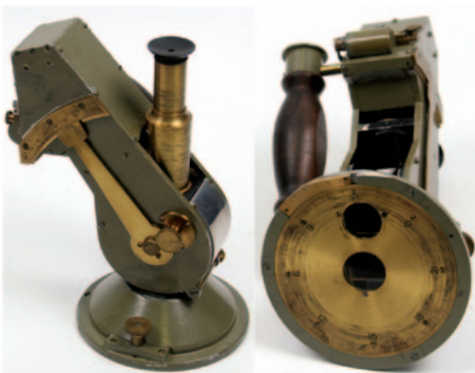
Figure 3 — Side (L) and bottom (R) view of a prototype model of Frank Hogg’s two-star sextant manufactured at the David Dunlap Observatory, circa 1940.
