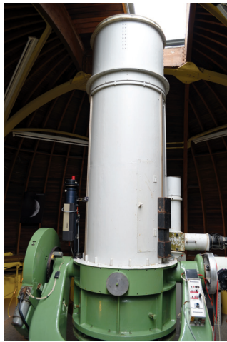
Figure 3 — The Waltz reflector of the Landessternwarte Königstuhl, with 72-cm mirror by Carl Zeiss, Jena. The telescope has an f/3.9 primary mirror. Its light-gathering power, although with a smaller field of view than the Bruce astrographs, made it ideal for asteroid followup after its construction in 1906. The telescope has been converted to a Nasmyth-Cassegrain with a secondary mirror near the entrance (top) and a tertiary mirror directing light to instruments along the declination axis (lower right). Photo by author.
