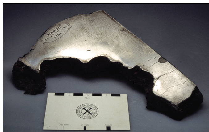
Figure 2 — An etched slice of the meteorite showing its name, date of discovery, and the supposed coordinates of its find. The meteorite's Widmanstätten structure is clearly visible. Curiously, the minute values of the find coordinates are reversed in Grady (2000) and the derived Meteoritical Bulletin on-line database, where they appear as 44°30'N, 77°28'W, a point near the junction of highways 7 and 62, on the north side of the town centre. Natural Resources Canada, Earth Sciences Sector photo No. 2006-096.
