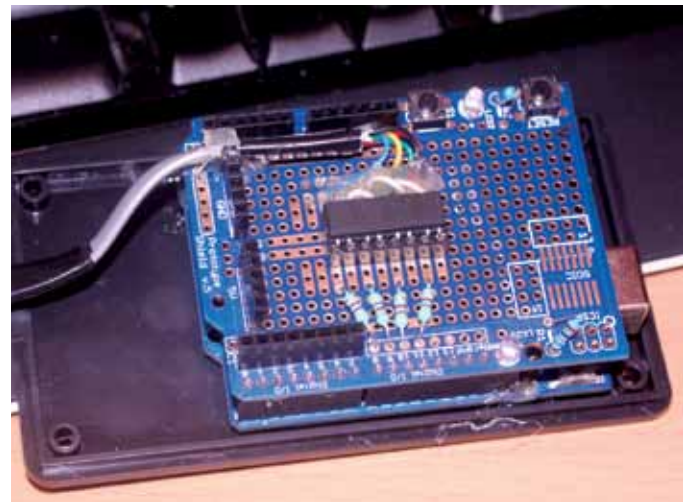
Figure 4 — The top of the prototype shield after wiring.
