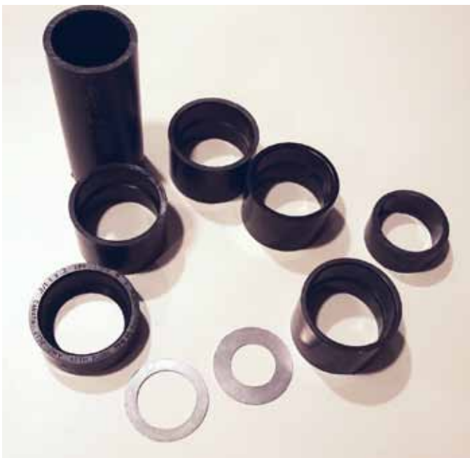
Figure 3 — ABS plastic components of the telescope baffles.
