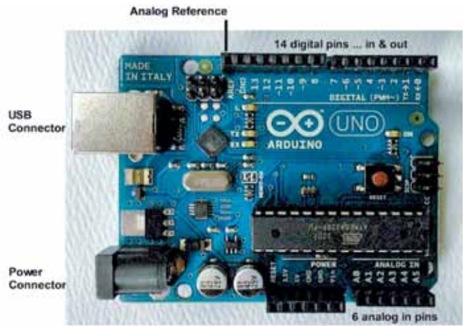
Figure 1 — The Arduino Uno with connections identified.
