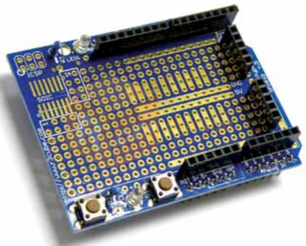
Figure 2 — The front of the Arduino prototype shield.
