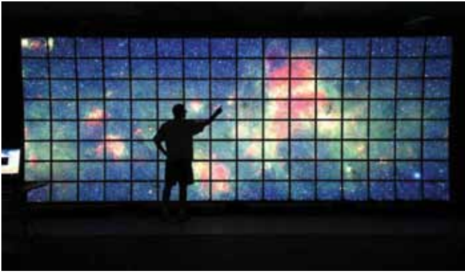
Figure 2 — Big Data on the Big Screen: The centre of the Milky Way galaxy, imaged by NASA's Spitzer Space Telescope, is displayed on a quarter-of-a-billion-pixel, high-definition 7-metre LCD science visualization screen at NASA/Ames Research Center in Moffett Field, Calif. Image: NASA/Ames/JPL-Caltech.
