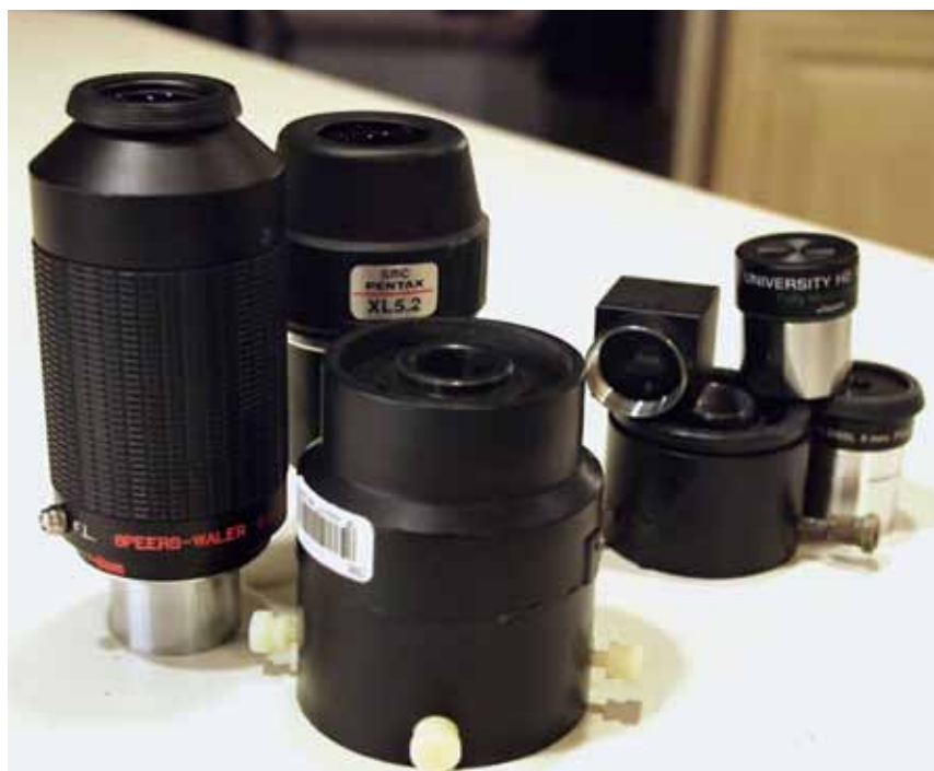
Figure 3 — The eyepieces used for eyepiece-projection imaging with a Flea CCD camera.
