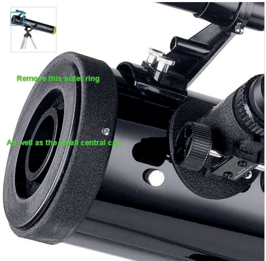
Figure 2 — I use this diagram to show telescope owners which caps to remove to use their telescopes.
