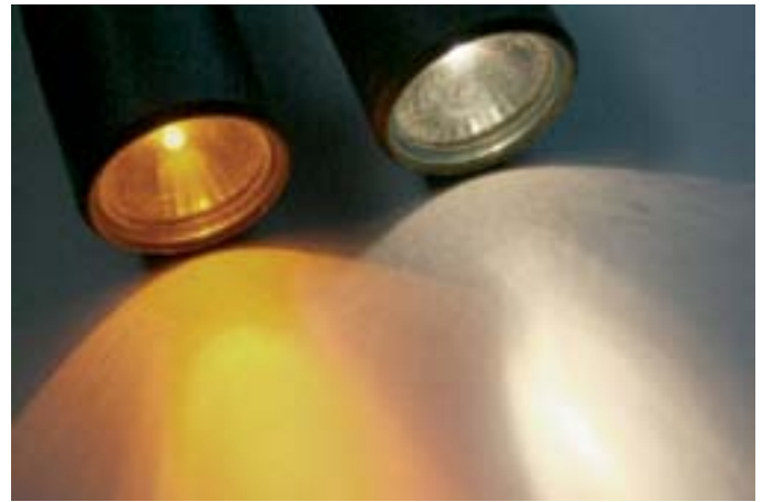
Figure 9 – A visual demonstration of the apparent colour difference between white and “true amber” LEDs. Most city dwellers are used to the amber colour from street lighting. “True amber” LEDs are readily available to flashlight manufacturers. However, most consumer flashlights are being sold with white LEDs, which are unsuitable for astronomy. The drive voltage for amber LEDs is about 3 volts so they may not require current-limiting resistors, except to reduce the LED brightness, which is considerable!
