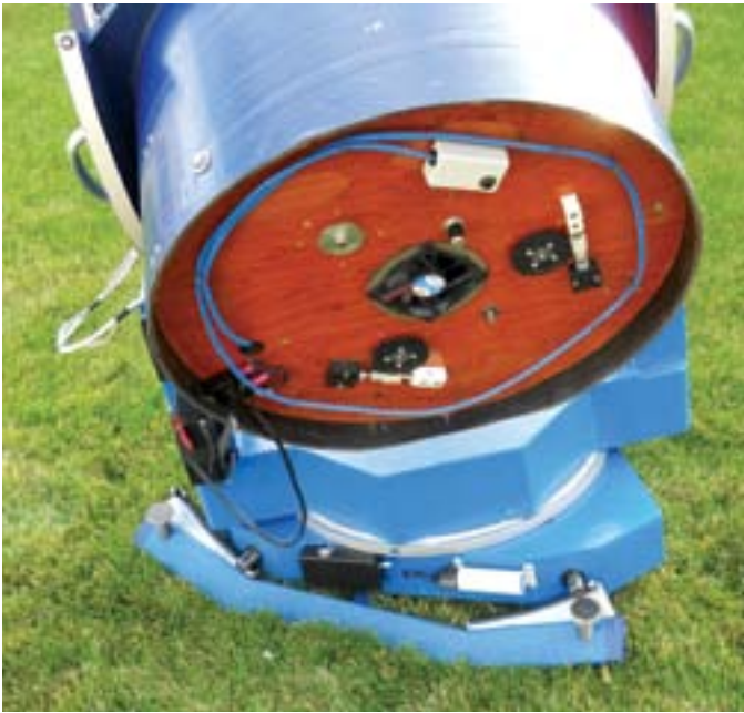
Figure 6 — Latest reincarnation with my T-bar EQ table, collimation drives, and ArgoNavis controller.
