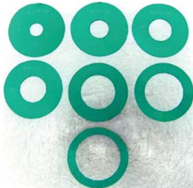
Figure 1 — Aperture stops AS1-AS7 (38.1mm-114.3mm; 1.5"-4.5") used on OTA1.
