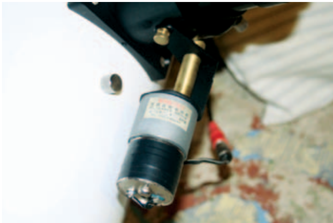
Figure 1 — The completed motorized focuser.
