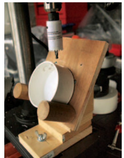
Figure 3 – The jig for drilling the hubs.
