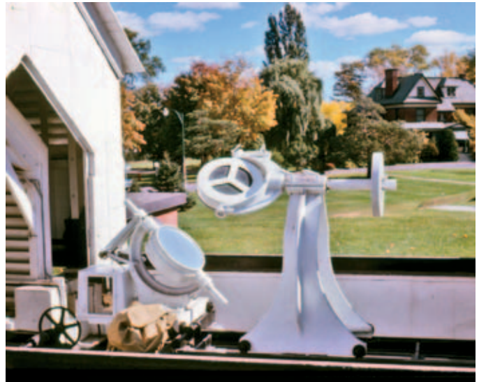
Figure 4 — Two plane mirrors of the three-mirror horizontal solar telescope, autumn 1963. The lower 24-inch mirror is mounted on an adjustable polar axis; it is the original coelostat purchased to observe the total solar eclipse of August 1905 in Labrador. The image-forming mirror is out of sight under the roll-back roof to the left. It reflects the beam, inclined slightly downward, to the right through a large opening in the casting that supports the upper plane mirror and toward a spectrometer housed in a basement laboratory. The Director’s House is in the background to the right.
