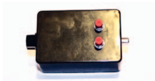
Figure 6 — The Hammond project box containing the focus-motor control electronics.
