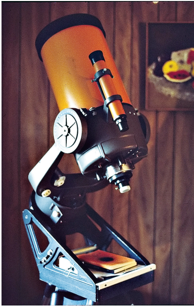
Figure 5 — The classic Celestron 10 Schmidt-Cassegrain (circa 1965 vintage) as it appeared in 1980, fully refurbished, painted, and mounted on a C14 wedge and tripod. Only about 300 of these superb f/13 telescopes were made.
