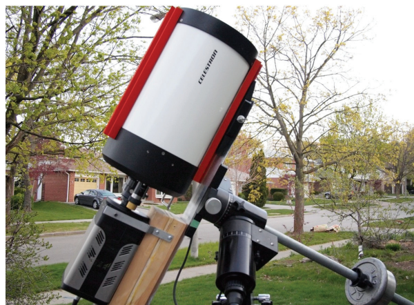
Figure 2 – The long mounting plate (a) needed to adapt the camera to the Celestron telescope (b).
