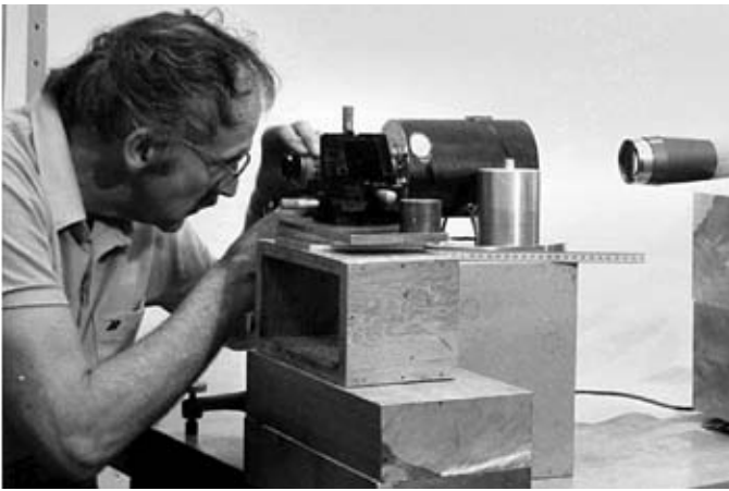
Figure 5 - Harvey making critical adjustments to a Viking Ultra Violet Imager for the mapping of dayside aurora from Earth orbit.
