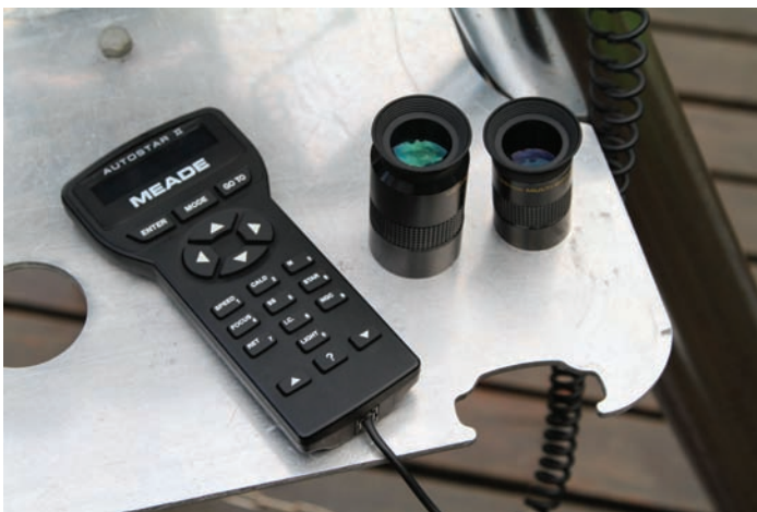
Figure 2: The hand-paddle slot is the trickiest bit; beaver out the material very slowly by moving the jigsaw side to side, checking the fit as you go. Finish the edges with files and sand paper.
