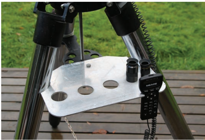
Figure 1: The tray has both 1 1/4" holes and 2" holes for eyepieces. The bolt at the back extends through a hole drilled into the spreader for the purpose and has a wing nut on the underside.
