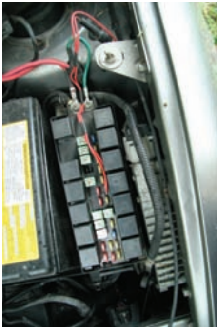
Figure 1 — The fuse box in a 1999 Dodge minivan. The large black squares are relays. Leave them alone. The smaller rectangles are high-capacity fuses. Leave them alone too. The much smaller coloured rectangles with numbers on them are the fuses. Find out which circuits they protect from the diagram on the lid or from the owner's manual. The daytime headlight fuse in this car was replaced by a switch with wires soldered to the tangs of a fuse and inserted into the socket. Such a circuit must be equipped with an in-line fuse.
