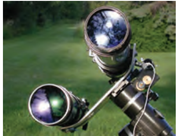
Figure 3 — The purple and green of modern coatings might allow brighter images than the older bluer coatings.
