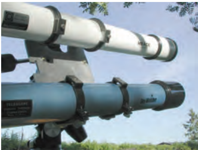
Figure 2 — The hinged rings of the newer scope are much more convenient and versatile.
