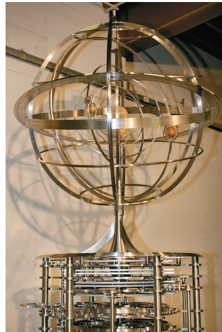
Figure 2 — The Long Now Orrery. Standing some eight feet tall, the orrery displays the relative positions of the planets Mercury through to Saturn. This image is just one of the 125 photographs taken of the orrery by Jake Appelbaum at its recent unveiling. The other images can be viewed at www.longnow.org/projects/clock/orrery .
