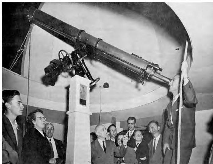
Figure 1 — The Montreal Centre's 6.5-inch f/15 Topham refractor with its setting circles.
