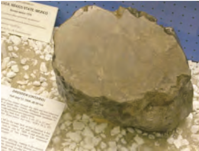
FIGURE 1 —The Dresden (Ontario) 40.01 kg main mass, with cut face displayed. The meteorite's dark fusion crust is ~1 mm thick and well-preserved. Internal brecciation is clearly visible, defined by dark hairline fractures which envelop centimetre- to decimetre-size chondritic clasts. Width of the cut surface is 32 cm.
