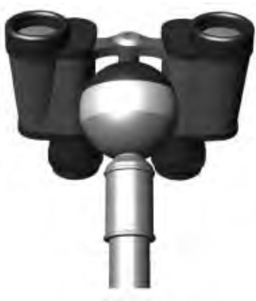
Figure 1 – A view of the binocular rest in operation. The rubber ball is attached by inserting the threads on the head of the pole sander into a deep "X" cut into the ball.
