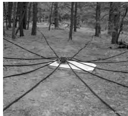
FIGURE 6 – A deployed infrasonic detector system showing noise-reduction hoses. Additional information and images can be found at aquarid.physics.uwo.ca/~pbrown/infrasound.htm .
