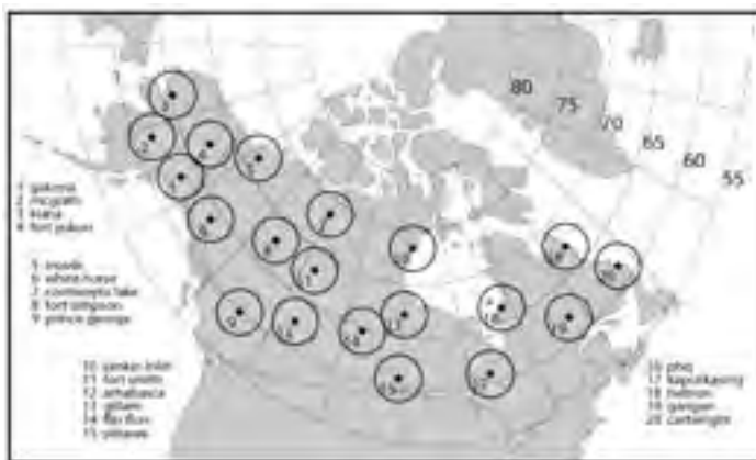
FIGURE 12 — THEMIS ground station coverage of Canada and Alaska. Much of Canada will be covered with imagers taking exposures every five seconds at night, with the data centrally accessible in real time. This should produce useful data for determining orbits and fall zones of bolides, in addition to the main aim of recording details of aurorae on a continental scale. Station names are shown around the map with numbers corresponding to those on the map. In all cases the station names correspond to those of the nearest geographical location: for station pbq this is an abbreviated form standing for Poste de la Baleine, Québec.
