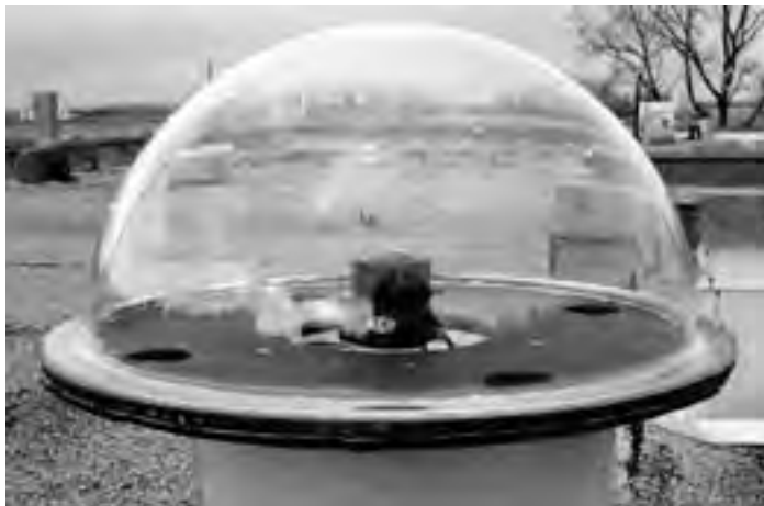
FIGURE 11 — Upward-looking Rainbow lens system under a clear dome, as installed in the University of Western Ontario bolide network.
