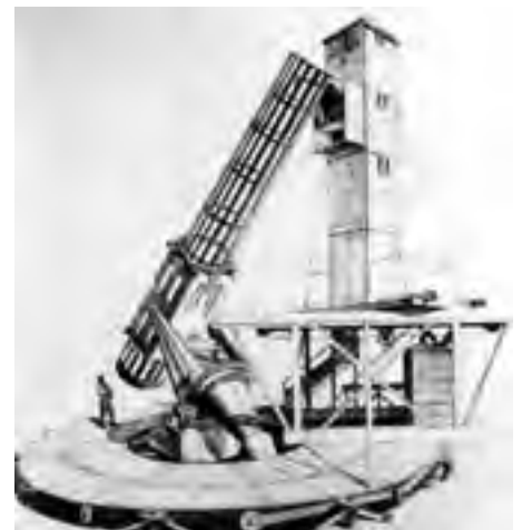
William Lassell's 48-inch equatorially-mounted reflector as it appeared in the year 1861. From The Victorian Amateur Astronomer .
