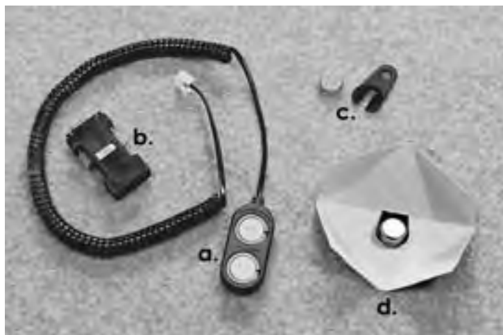
a) Blue Dot Receptor (dual) with cable; b) Universal Serial Adapter; c) iButton and flanged fob; d) iButton in fob, mounted in an "awning" cover."
