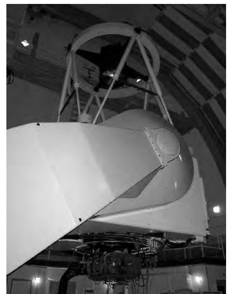
The 2.5-metre (100-inch) Irénée Du Pont Telescope at Las Campanas Observatory. Image from, and more information at, www.lco.cl/lco/telescopes/duPont
