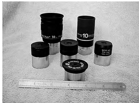
Front Row: Orthoscopic. Middle Row left to right: No-name Plossl, Antares Ultima Plossl, No-name Kellner. Back Row left to right: TeleVue Radian, Vixen Lanthanum.
