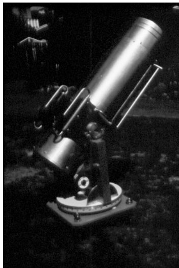
The 32-cm f/4 reflector, with stainless steel tube and mount, used to make the grand tour of the Southern Skies in New Zealand.
