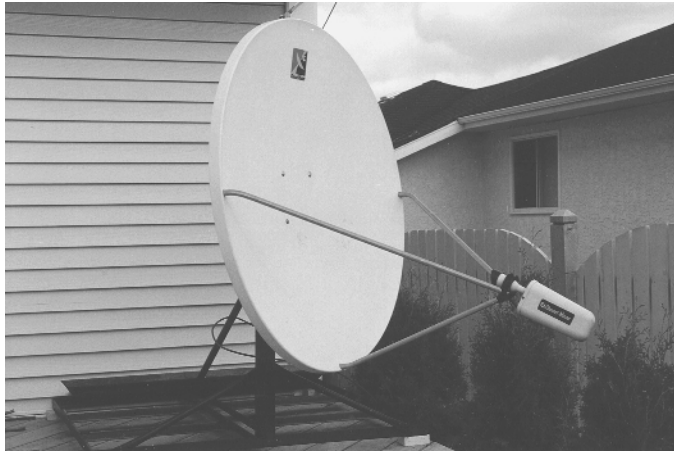
FIG. 2 — The 1.2-metre dish antenna and the block diagram of the Radio Telescope.
