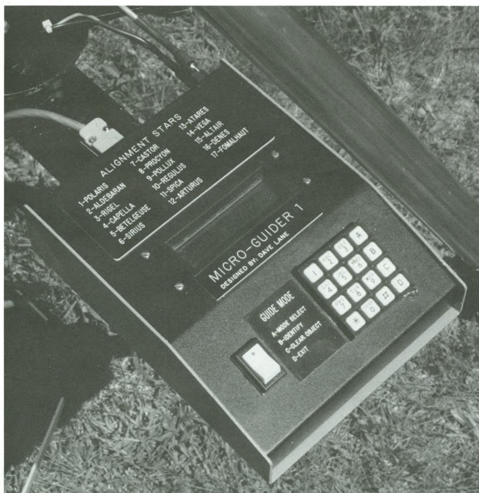
A close-up view of the Micro-Guide. Note that for entering negative declinations the "D" key is used as the keypad has no minus key. Photo by the author.
