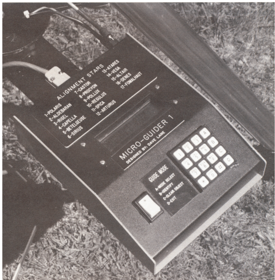
A close-up view of the Micro-Guide. Note that for entering negative declinations the "D" key is used as the keypad has no minus key. Photo by the author.
