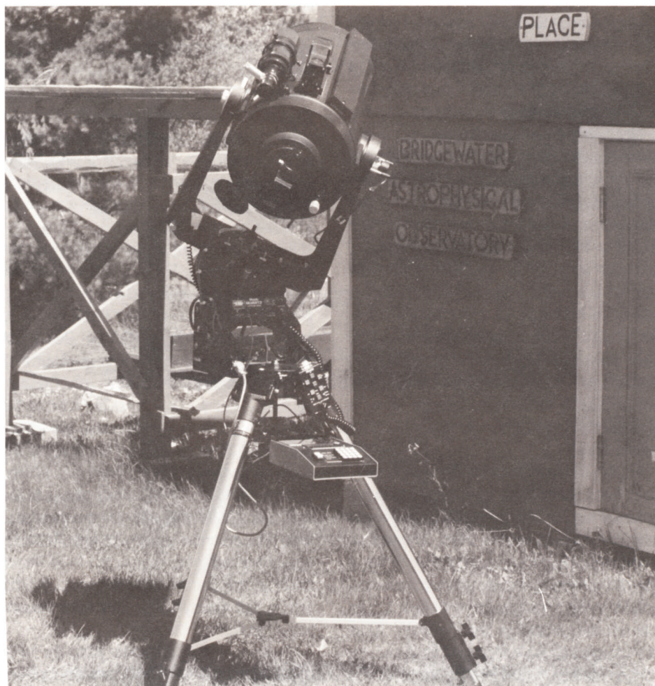
The Micro-Guider, shown attached to the author's Meade 2120 telescope. Photo by the author.
