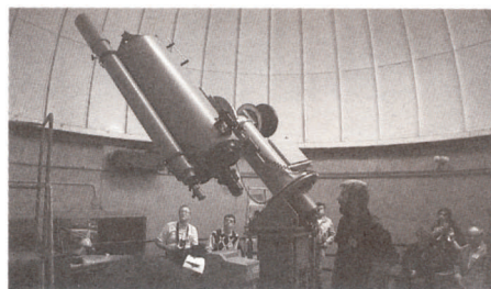
The workings of the 20" f/15 Cassegrain telescope at the Gordon Southam Observatory are being demonstrated by Dave Dodge
