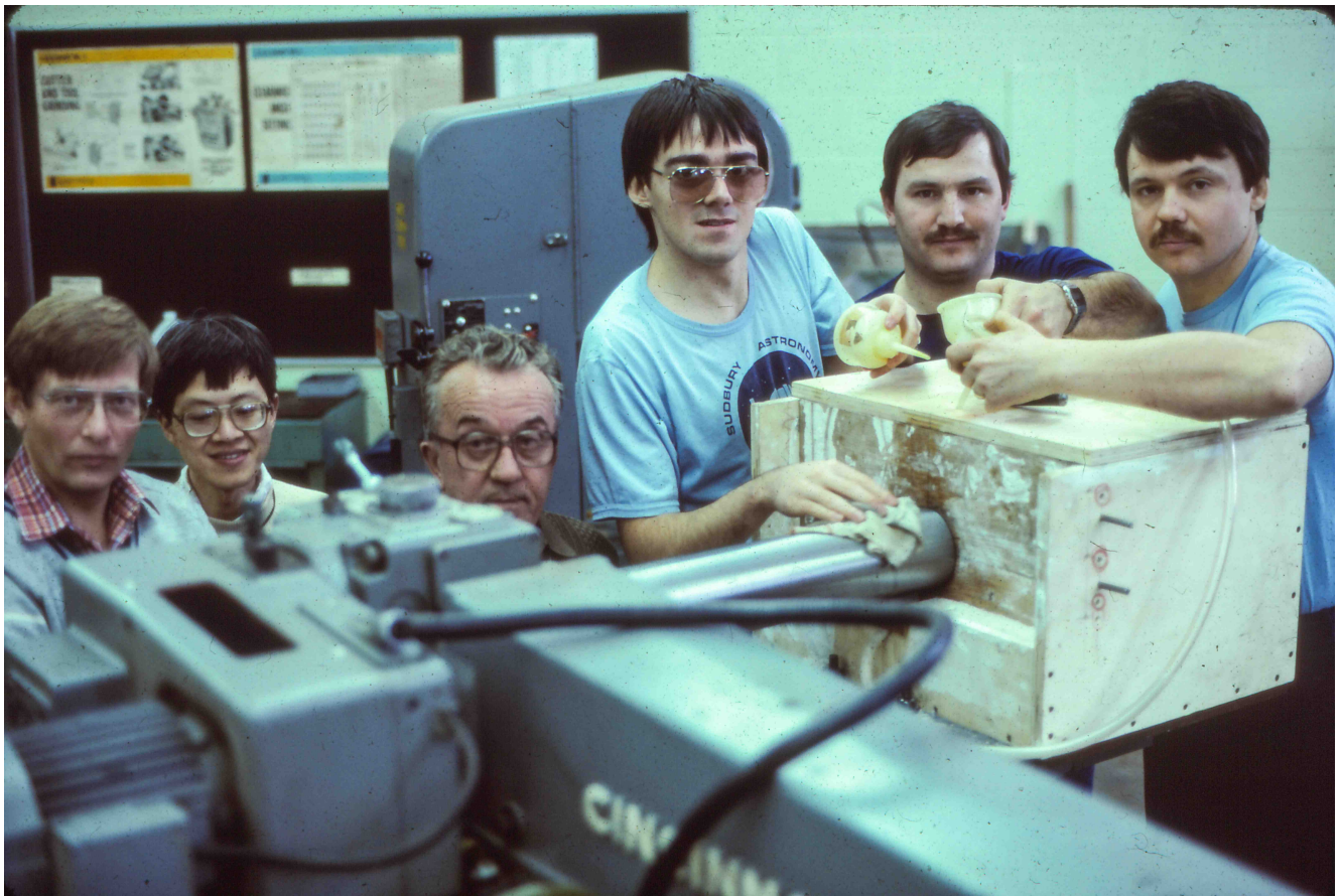
18 - 726 (December 10, 1983) The Guide Box and Flat have been Mounted on the Lathe, and the spinning coring tool has started to penetrate the Glass. Ken Odasky is keeping a careful watch on the process. Wilf Meyer is in the left foreground and Alan Ward is in the background adding cutting fluid.
