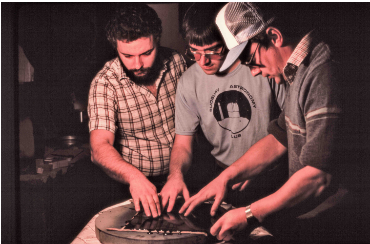
13 - 724 (late Nov. 1983, BELOW) Flat Placed in Guide Box for Boring. Notice the white tube near the Center of the Flat, which will guide the Boring Tool.
