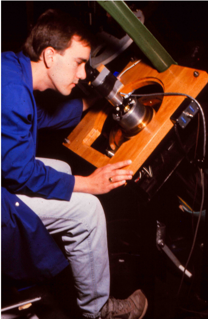
53 - 1222 (August 1985) Pierre Harrison is Observing the Sun in Hydrogen-Alpha Light. The eyepiece he is looking into is at the end of a slanted 10-foot-long Telescope Tube that extends downward through one of the Beam tubes to a 4-inch Flat Mirror outside the building. The Drive Gear is just below the oak face plate of the Telescope.
