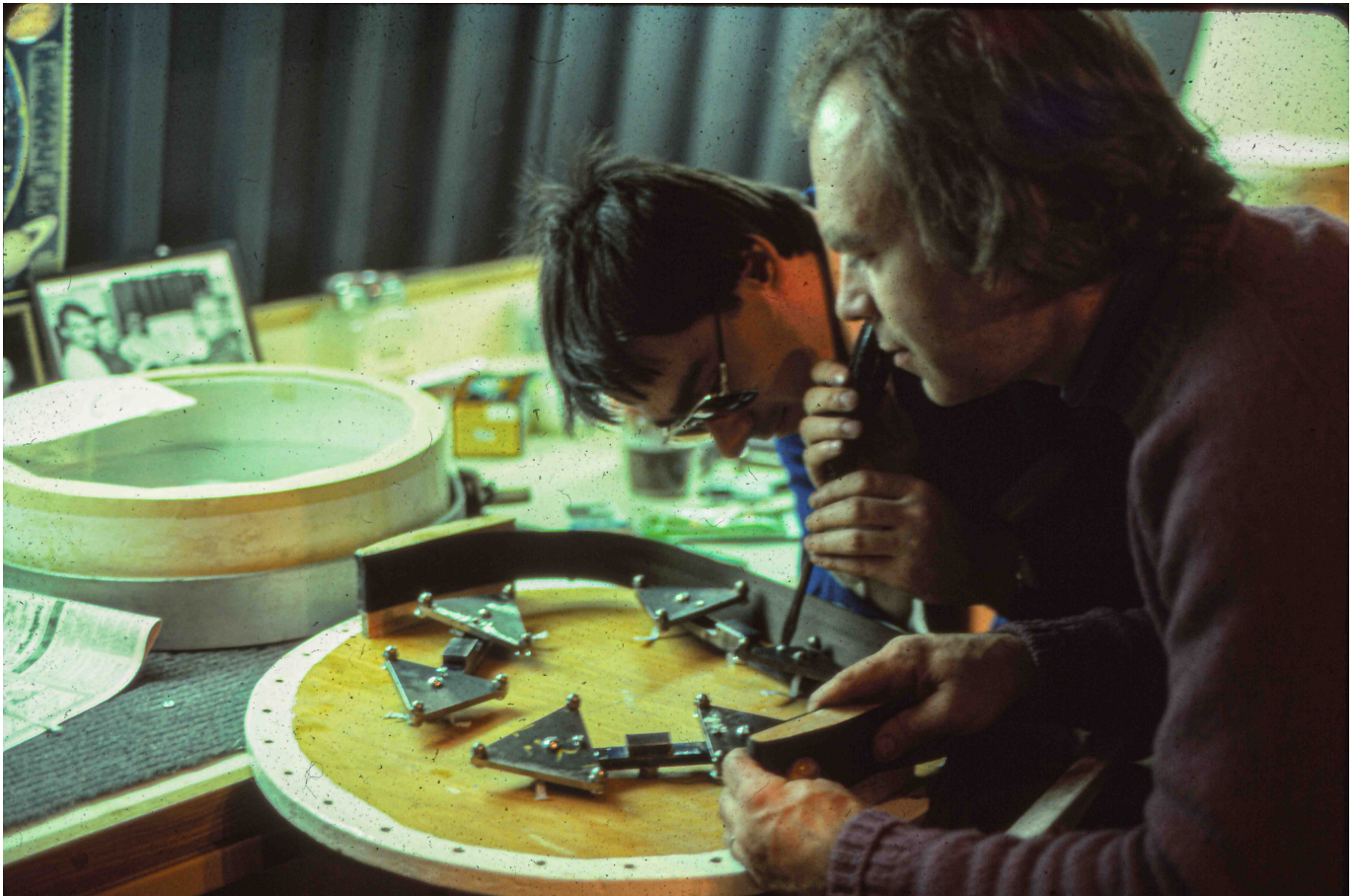
34 - 850 (February 1985) In the Optical Workshop on the 4th Floor of Science North, Steve is seen with Alan Ward assembling the supporting structure of the Mirror Cell for the Concave Long-Focus Primary Mirror, which will form the light from the Perforated Flat Mirror into an image of the Sun.
