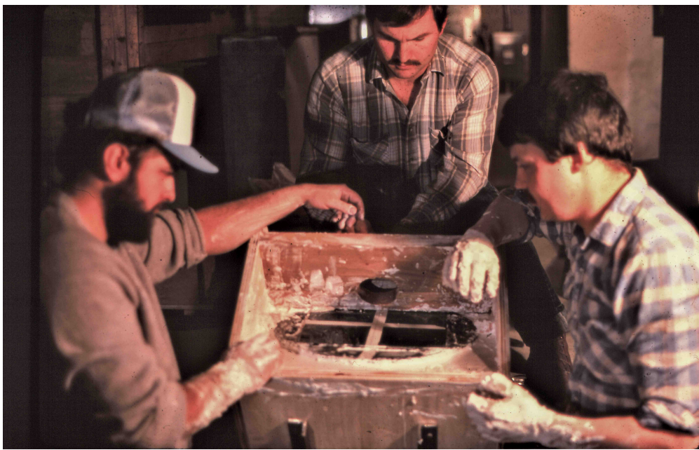
14 - 723 (Late November 1983) Securing the Flat in Plaster for Boring... (left to right) Greg Beach, Gerry Bourque, Carl Hoeg
