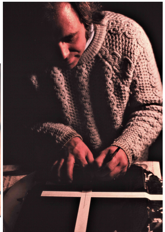
13 - 724 (late Nov. 1983, BELOW) Flat Placed in Guide Box for Boring. Notice the white tube near the Center of the Flat, which will guide the Boring Tool.
