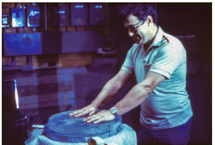
(Bottom:10 - 709, July 1983) Fred Pushing Glass. Grinding is a mostly back & forth motion.
