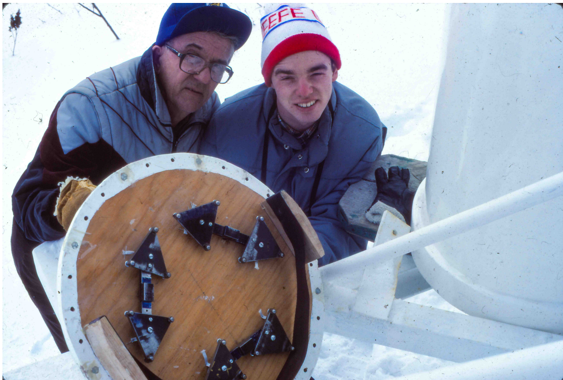
35 - 852 (February 1985) Ken Odaisky and Gerhard Schinko are installing the Mirror Cell on the Triangular Base Frame at the Bottom of the Polar Axis.
