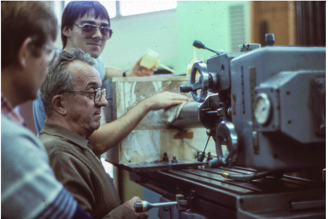
18 - 726 (December 10, 1983) The Guide Box and Flat have been Mounted on the Lathe, and the spinning coring tool has started to penetrate the Glass. Ken Odasky is keeping a careful watch on the process. Wilf Meyer is in the left foreground and Alan Ward is in the background adding cutting fluid.
