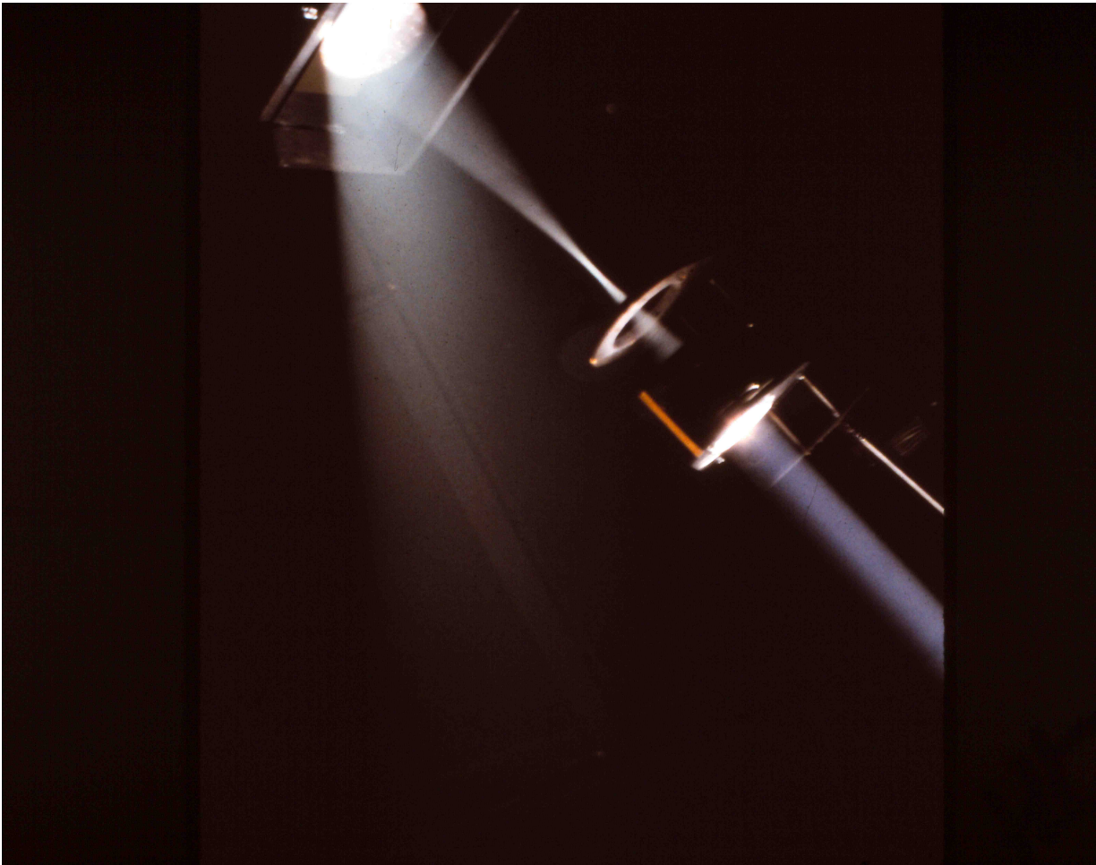
41 - 1152 (February 1985) The Beam of Sunlight seen on the previous page now passes through an imaging lens (an aerial camera lens which I brought back from the Stellafane Telescope-maker's Convention in Vermont). The expanding cone of light is then directed downwards to the large Rotating Screen by the Plane Mirror at the top.
