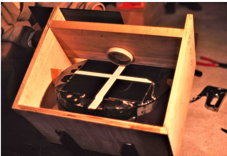
13 - 724 (late Nov. 1983, BELOW) Flat Placed in Guide Box for Boring. Notice the white tube near the Center of the Flat, which will guide the Boring Tool.
