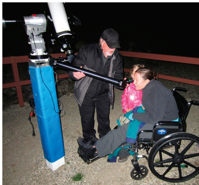
Member Guy Mackie with our Astrophysics 5.1 Telescope and new Articulating Eye Piece providing a direct look at a celestial wonder to an appreciative visitor at the Okanagan Observatory on one of our numerous Friday Public Nights
